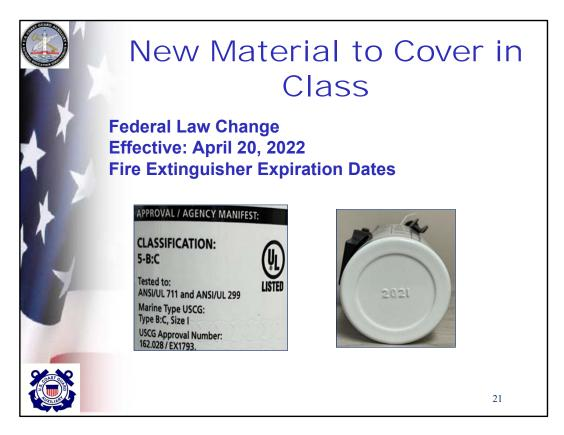
If a fire extinguisher has a date of manufacture stamped on the bottle (example: "05" means 2005), and it is older than 12-years old, the extinguisher is considered to be expired and must be removed from service. Look for wording on the bottle stating "This product must be removed from service within 12 years after the date of manufacturing".
